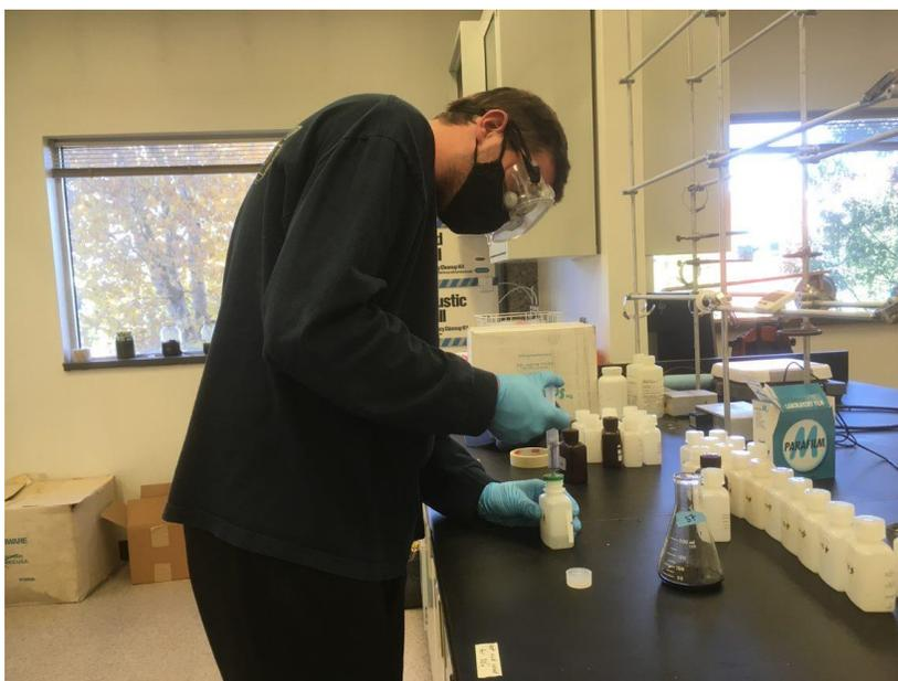
Figure 2. Filtration of sample water after biochar treatment.
