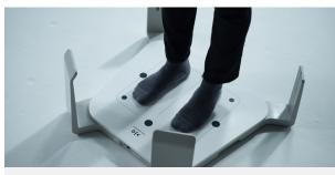
Scan / A 3D scanner captures 16 key foot measurements, and a pressure plate visualizes gait and pressure points.
