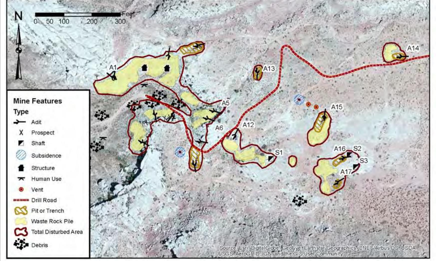
Figure 2 - Physical features at the Telluride 18 mine site. Adits, prospects, and shafts are numbered. Mine entry features that are labeled (e.g. 'S1') are open.
