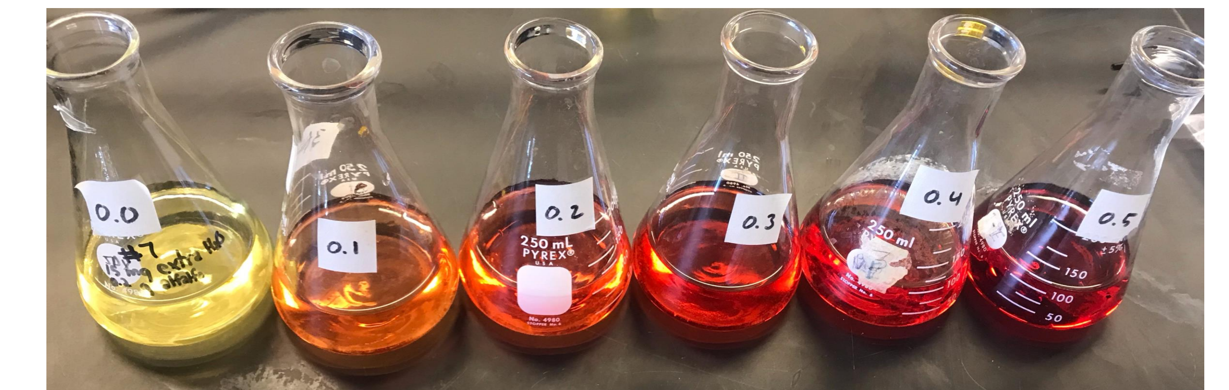
Known concentrations of phenol with color indicator used to create the calibration curve
