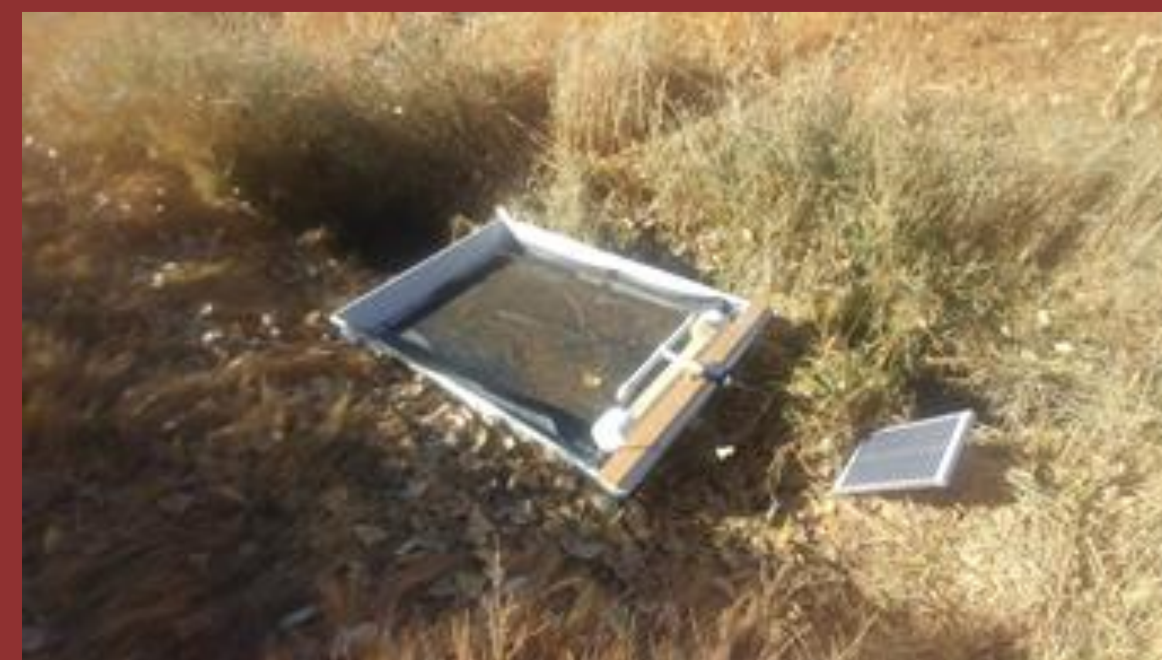
Fig 1. Picture showing pilot-scale (ATST ™ ) system in place running water. Water is pumped and returned in to a continuously flowing irrigation outflow.
