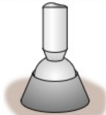
ball stays in socket & is free to rotate
