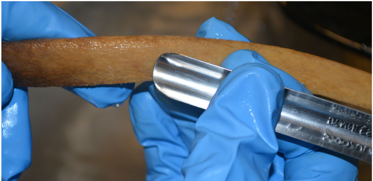
Figure 13: Mechanical tissue removal using scoopula; note the parallel position of the tool.
