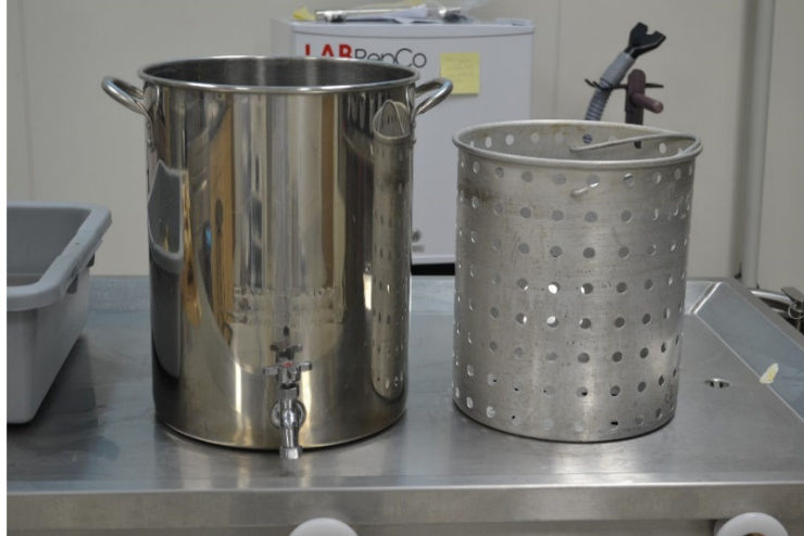
Figure 8: Boiling pot and strainer; fill the strainer with long bones prior to submersion in the pot.
