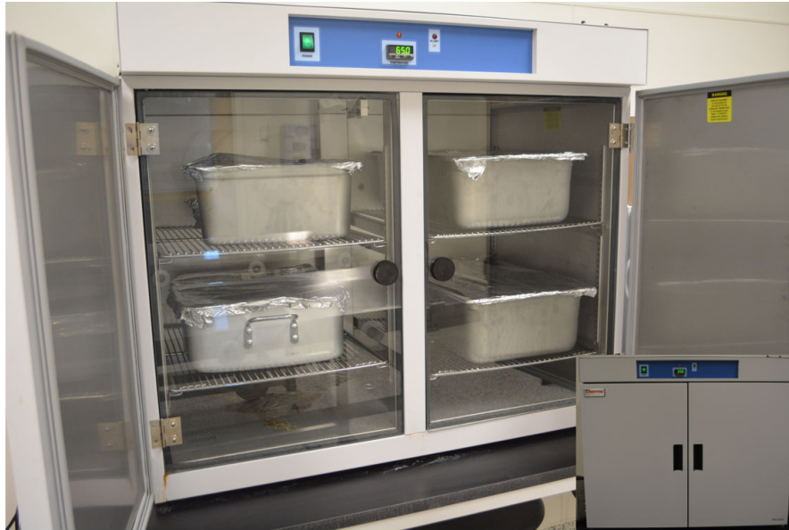
Figure 6: The incubator, with pans covered with aluminum foil and set to 65 Celsius.
