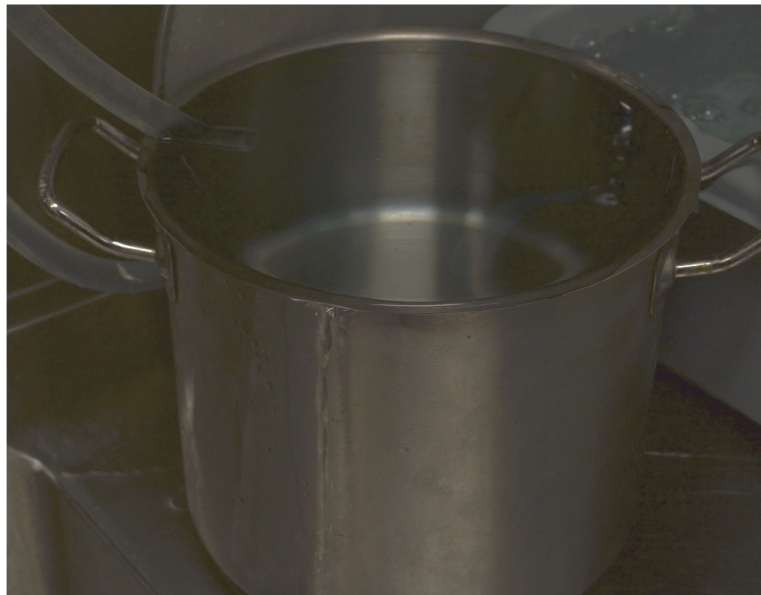
Figure 23: Correct level of water overflow in preparation for fresh water stop bath
