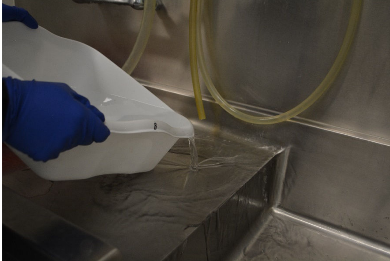
Figure 22: Technician discarding the ammonia bath in preparation for the fresh water stop bath.
