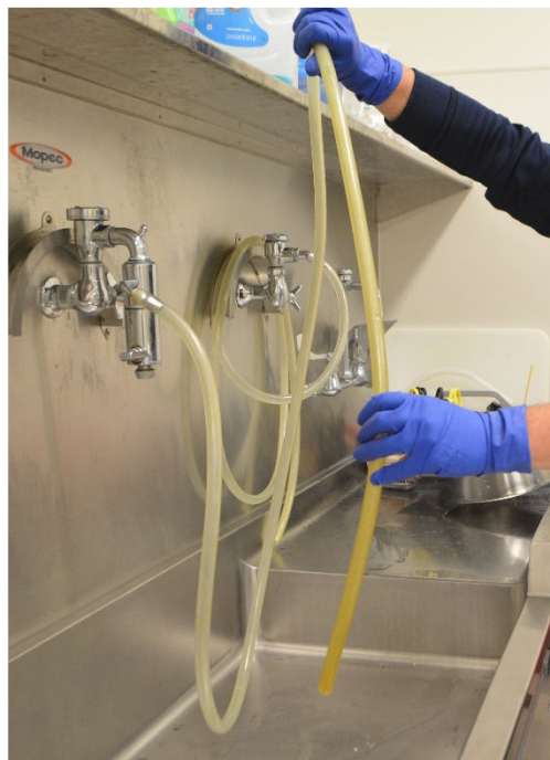
Figure 32: Drain hose of residual water before re-hanging
