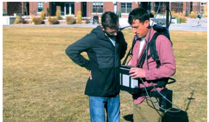
Geoscience students Ryan Mumby (left) and Evan Pellowski (right) check magnetic readings on the GSM-19TW.
