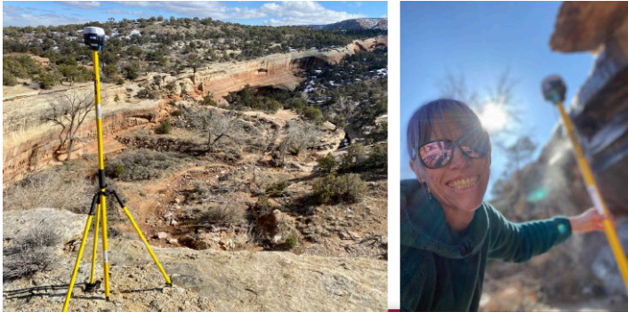
Dr. Kerry Riley and RTK GPS equipment that she is using in her classes.
