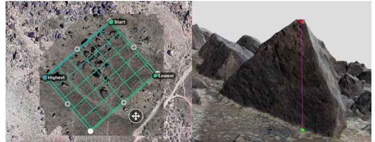
Brauch to determine the accuracy of boulder geometry and volume estimates from resulting 3-D digital models (right). Note, the image on the right is a digital model, not a photo.
